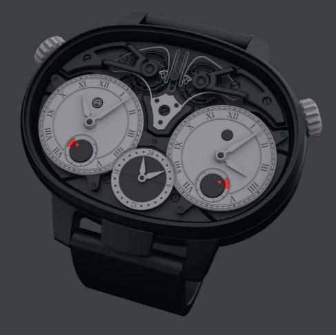
When fully wound, the watch has a 110h power-reserve. Some thirty turns for each movement are needed to wind the watch fully. Each movement is fitted with a slipspring, which is not locked when the movement is fully wound. You may also check the state of winding by looking the power re-serve indicators. The power reserve of a movement is low when the respective pointer faces the red sector as illustrated on the figure below.
