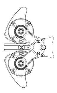
Resonance watches are so rare precisely because they are so extraordinarily difficult to design and produce, as they essentially require two watch movements to be combined into one unit that utilizes two independent mainsprings, gear trains, escapements, and balances. A resonance watch requires its two balance wheels find a concurrent rhythm so as to continuously regulate one another. The follow-on challenge is to consistently
