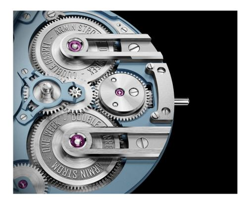
New movement, new beat rate. Another major evolution in the new One Week is the oscillating frequency of the regulating organ. As it is designed as an all-occasions watch that can take on dynamic activities, the beat rate has been increased from 2.5 Hz to 3.5Hz (25'200 vph). This higher frequency, which offers a more stable chronometric performance, required the entire gear train to be recalculated and reconfigured.
