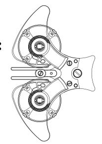
The twin balance wheels of the Armin Strom Mirrored Force Resonance oscillate in opposite direction. If you have not worn your watch for some time and restart it by manually winding it, the oscillators will synchronize in less than ten minutes. In case of a disturbance such as a shock, it takes only a few minutes for the two balances to find their resonant rhythm once again.
